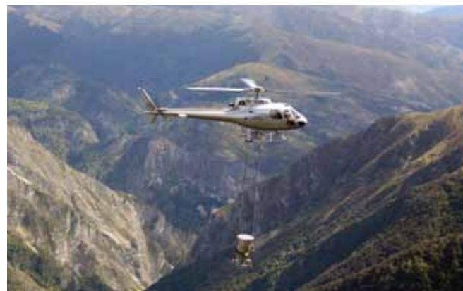
Figure 4. Typical helicopter and bait spreader bucket used in aerial rodent eradication projects.
